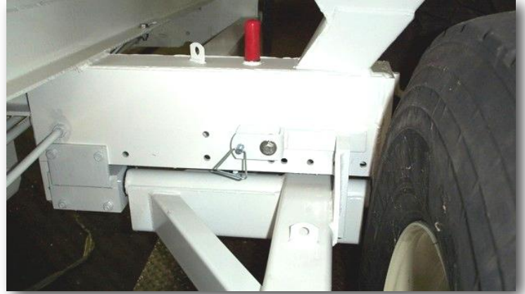
STOP BLOCK IN ENGAGED POSITION
